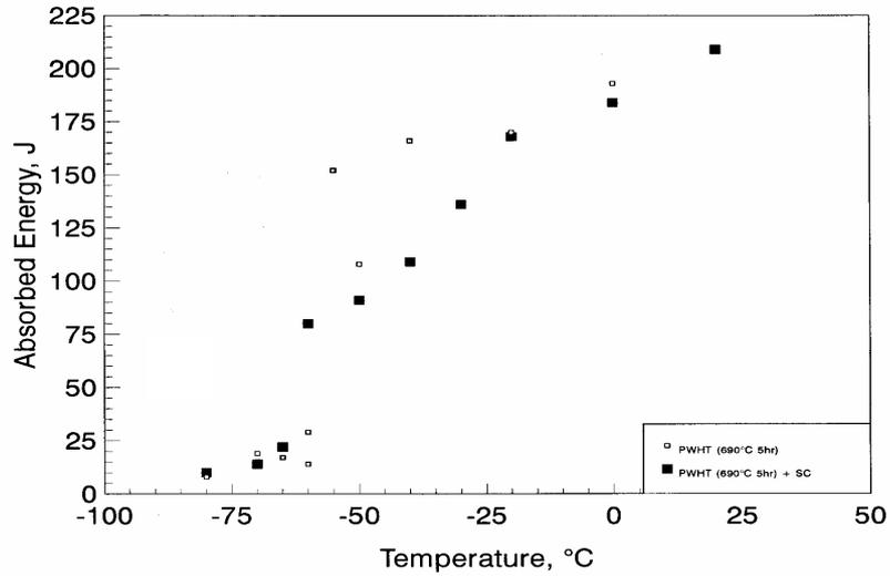
$T_1 = 54\text{J transition temperature after PWHT} = -58^\circ\text{C} (-72^\circ\text{F})$
