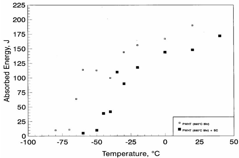
$T_1 = 54\text{J transition temperature after PWHT} = -59^\circ\text{C} (-74^\circ\text{F})$
