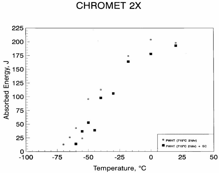
$T_1 = 54\text{J transition temperature after PWHT} = -54^\circ\text{C} (-65^\circ\text{F})$
